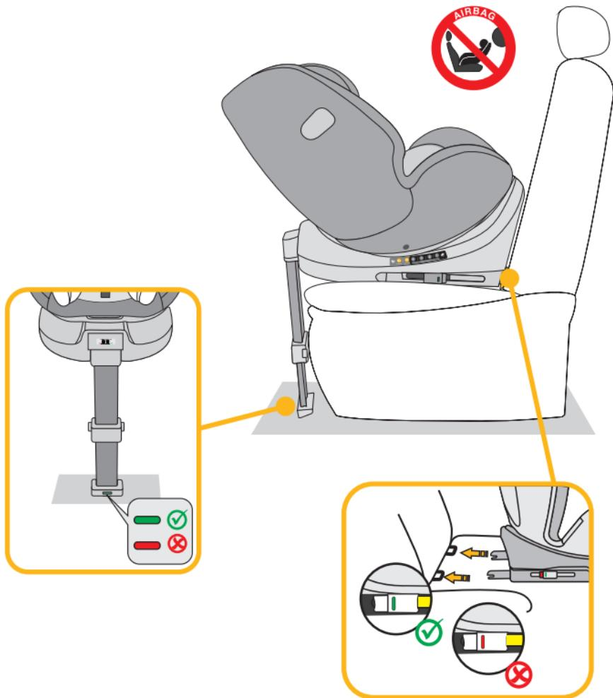
1. Adjust the child car seat to the maximum reclining position and turn it so that it points to the R1 – 40–75 cm seating position in rear-facing orientation. If your child's height exceeds 75 cm, please change to the seat position R2 – 76–105 cm.
