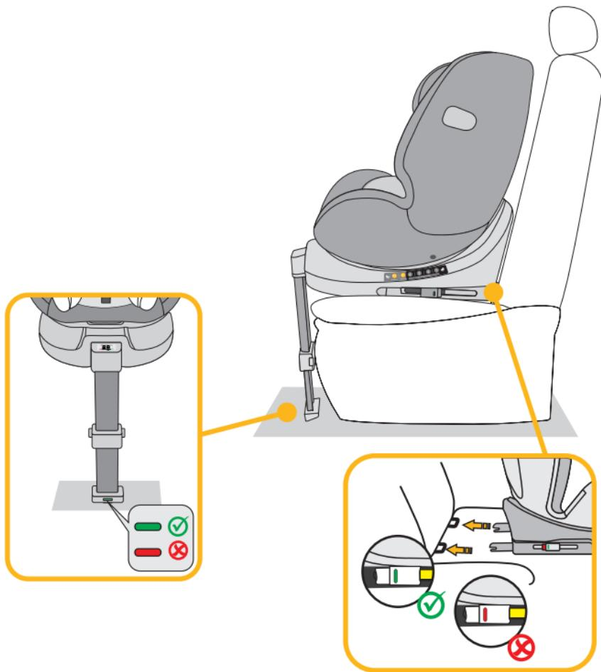
1. Press the two side Isofix connector buttons to extend the length of the Isofix connectors.
