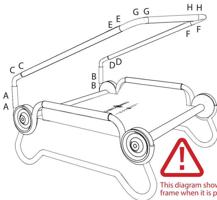
This diagram shows the Dog-Bed Canopy frame when it is properly assembled.
