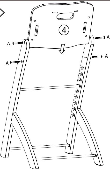
**EN** Important note for optimal stability: Only tighten all screws at the final step of assembly, with all 4 legs on the floor !
